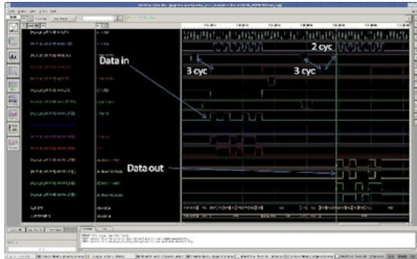
Figure 4 – Magma FineSim Pro screen shot showing results of memory block simulation.
